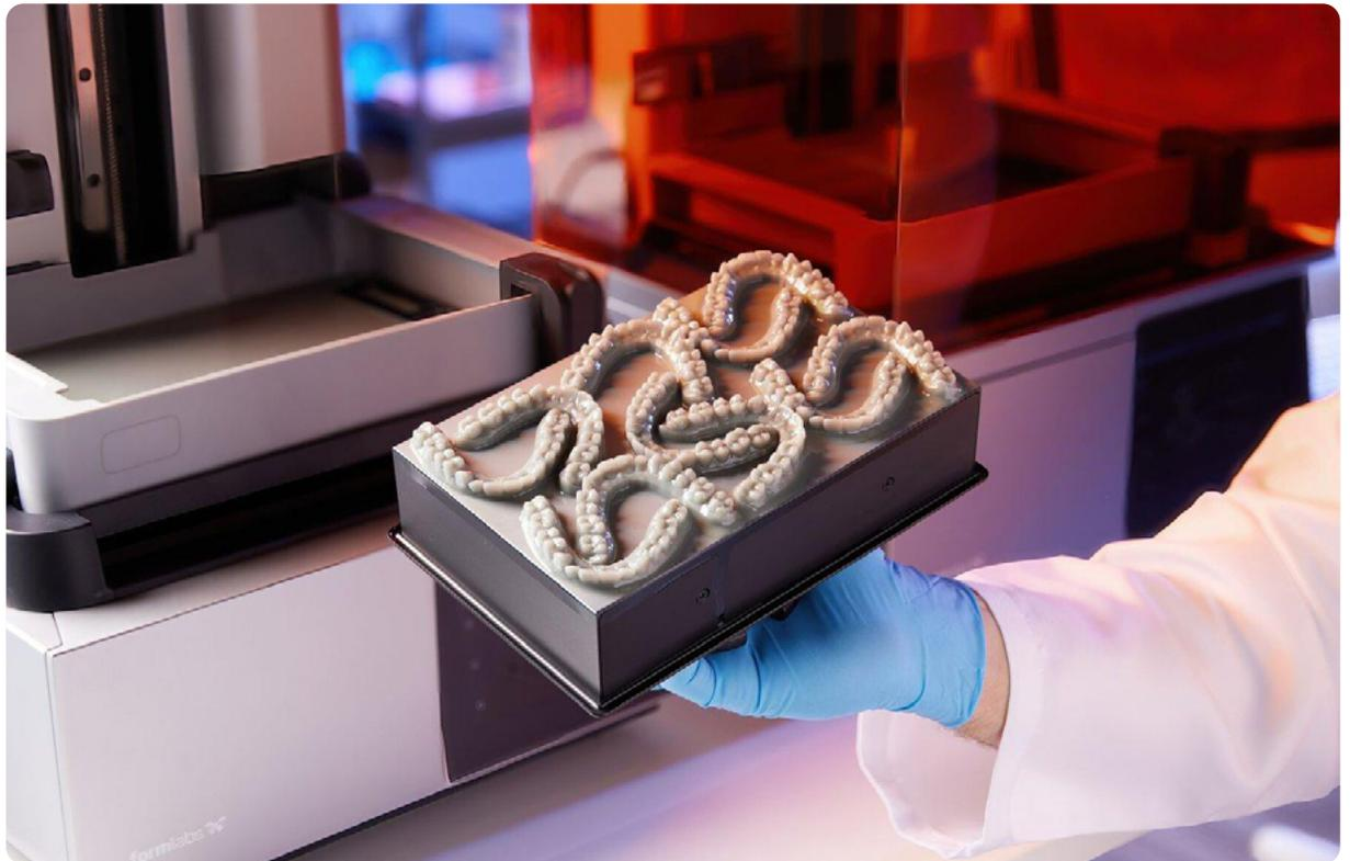
*With the LFD Print Engine of Form 4 Series printers, surface accuracy is over 95% of data points within 50  $\mu$ m of the original CAD data consistent across the build platform – while being able to print 11 models in nine minutes on Form 4B, and 32 models in 14 minutes on Form 4BL.*
