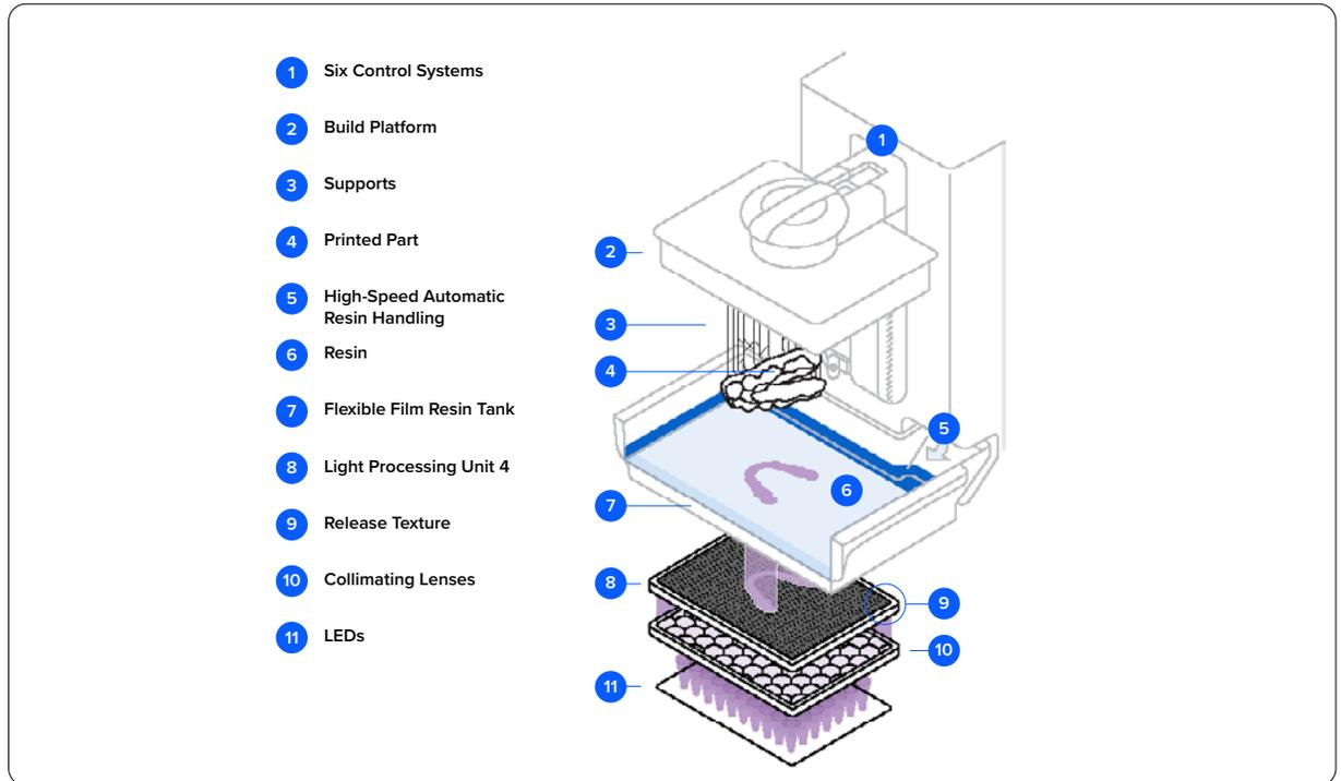
*The most common 3D printers for orthodontic applications work by selectively exposing liquid resin to a light source filtered and projected by various light-processing techniques to form very thin layers of material that stack up to create a solid object.*
