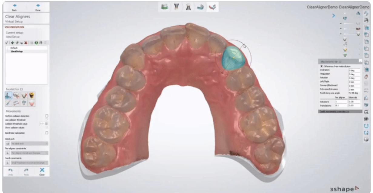
*A model for thermoforming aligners being designed in 3Shape.*
