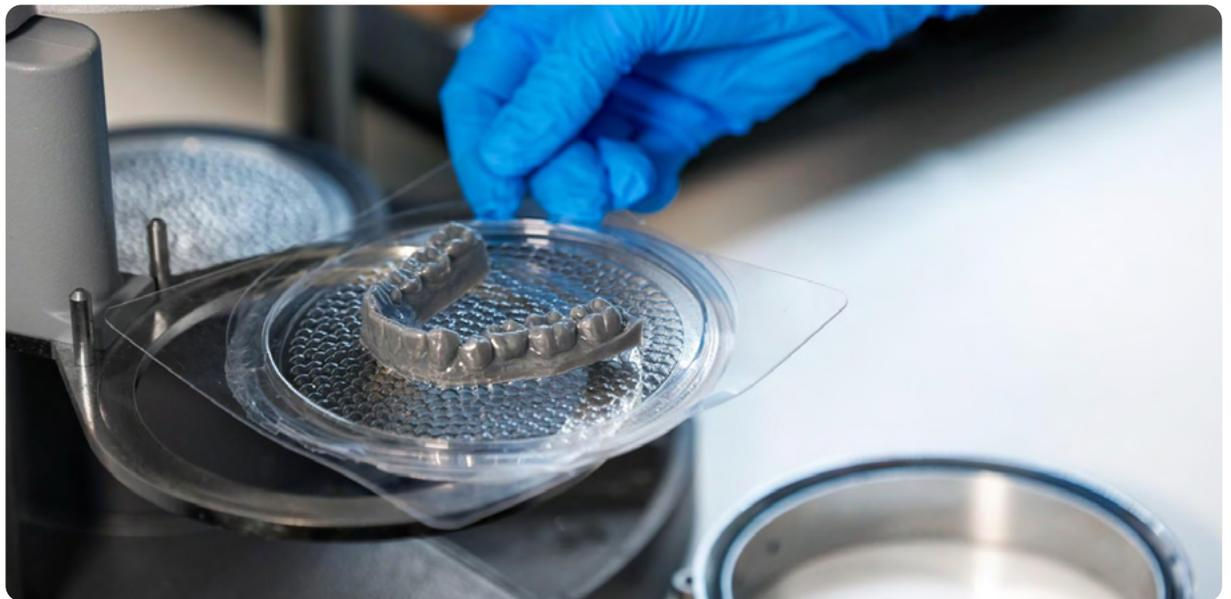
*Manufacturing thermoformed appliances like clear retainers and aligners over 3D printed orthodontic models is fast and affordable.*
